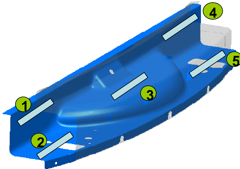
Figure 1: Tensile coupons cut out from the locations of interest for mechanical properties determination.
