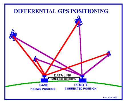
Figure 3. Differential Global Positioning System coordinates for precision mapping (Courtesy: Peter H. Dana, University of Colorado [9])
