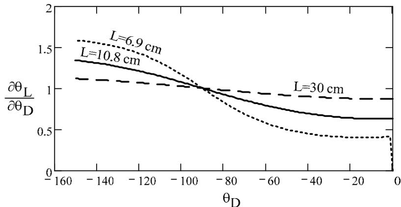
Figure 7.  $\theta_L$  sensitivity versus  $\theta_D$  for various arm lengths,  $L$ .
