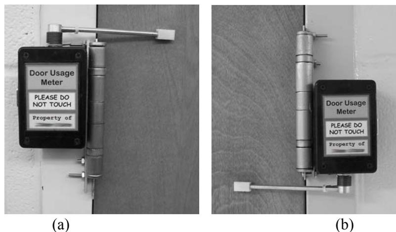
Figure. 2. Door monitor system installation on (a) right-hand and (b) left-hand swinging doors.
