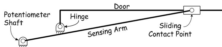
Figure 4. Linkage model of sensing arm and door.
