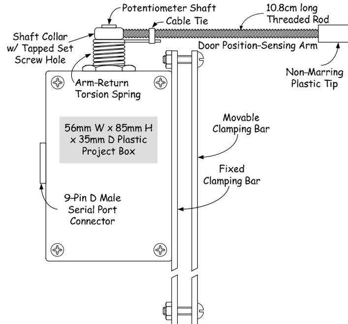
Figure. 1. Door monitor assembly drawing.
