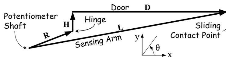
Figure 5. Vector model of sensing arm and door.
