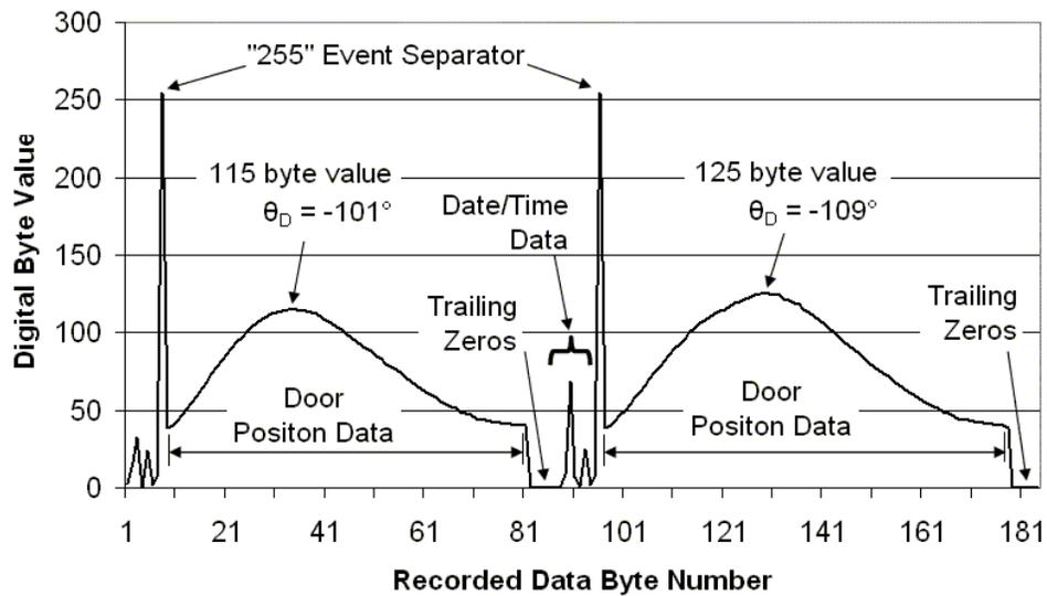
Figure 12. Plot of recorded door usage data for two consecutive door opening events.
