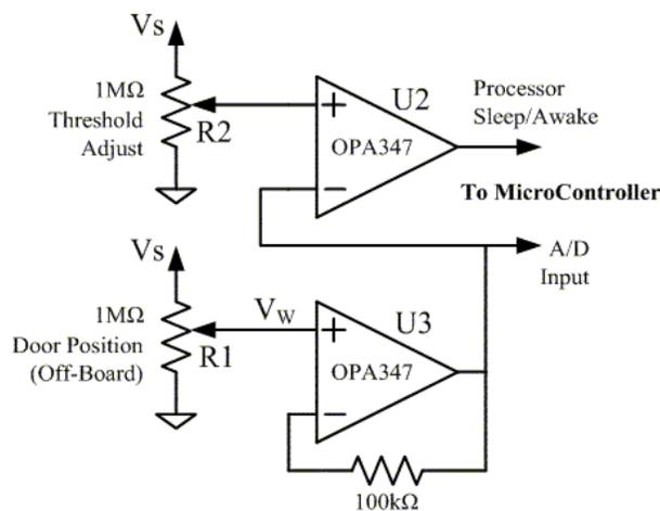
Figure 8. Buffer and comparator circuit schematic.
