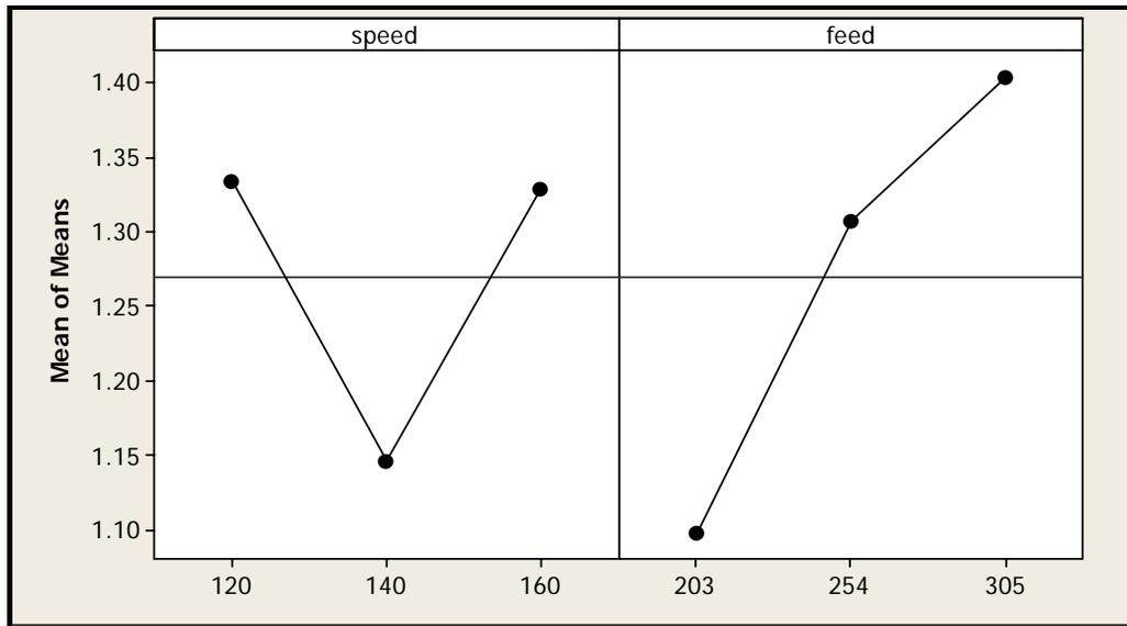
Figure 2:  $R_a$  Response Plot for 75% Phenolic Sample
