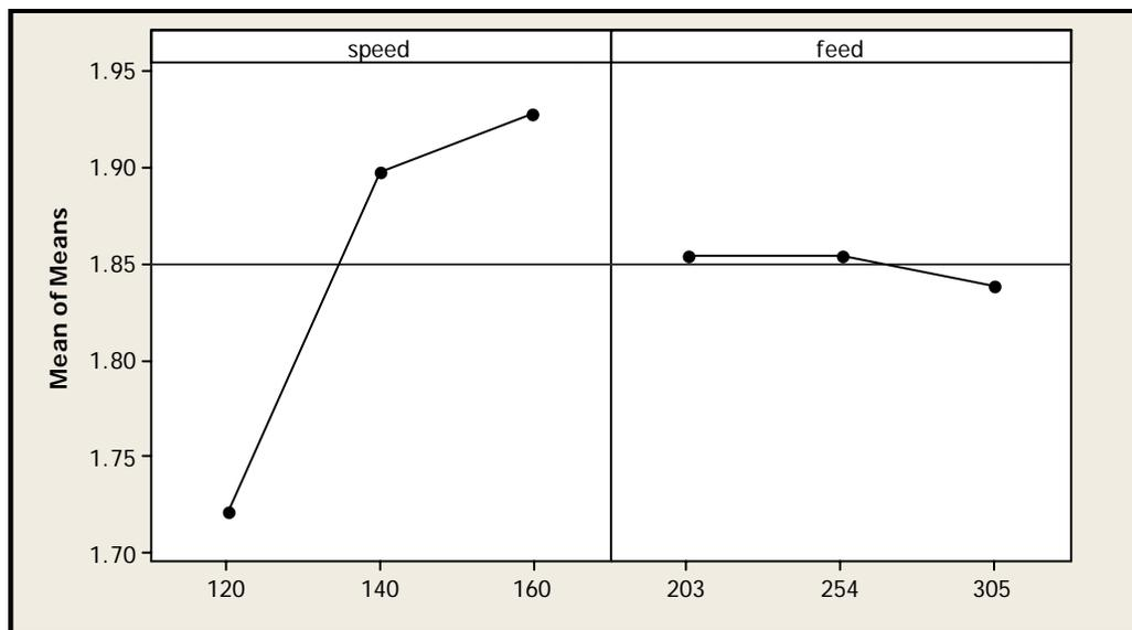
Figure 3:  $R_a$  Response Plot for 50% Phenolic Sample
