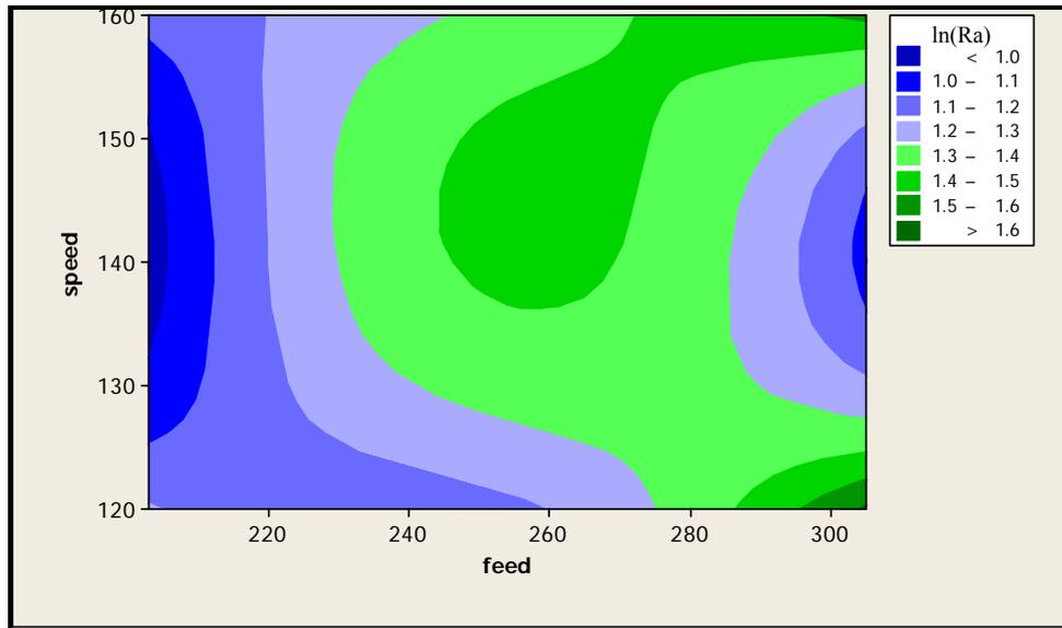
Figure 5: Contour Plot of  $\ln(R_a)$  vs. Speed and Feed - 75% Phenolic Sample
