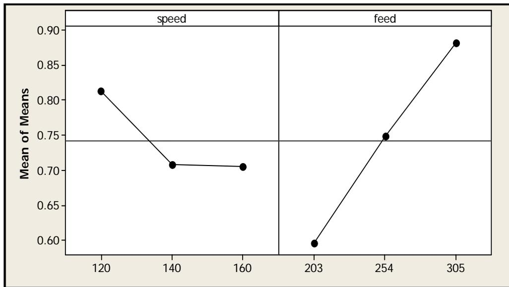
Figure 1:  $R_a$  Response Plot for 100% Phenolic Sample
