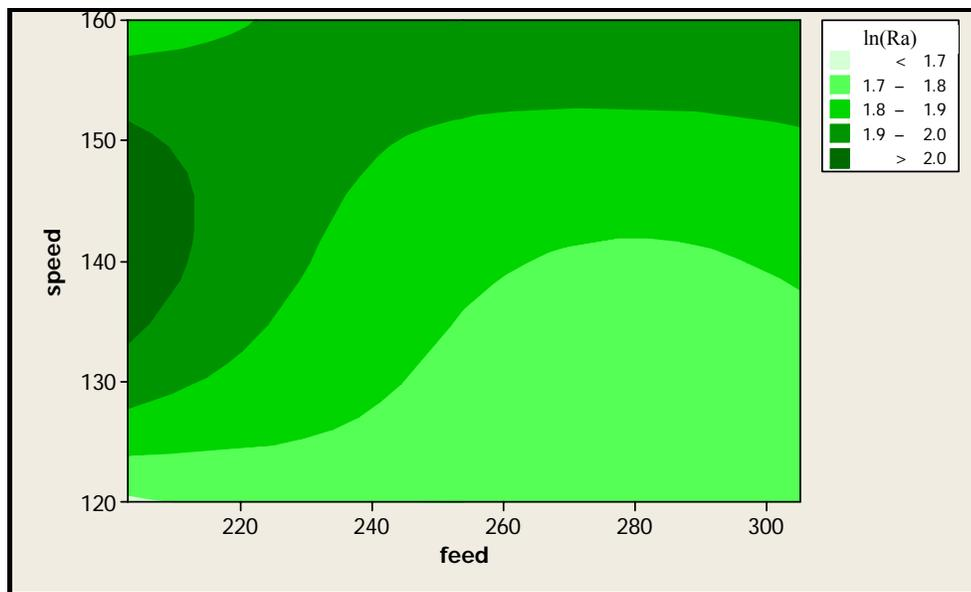
Figure 6: Contour Plot of  $\ln(R_a)$  vs. Speed and Feed - 50% Phenolic Sample
