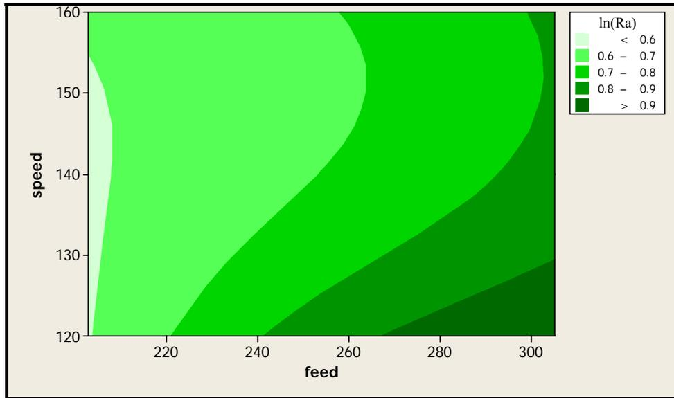
Figure 4: Contour Plot of  $\ln(R_a)$  vs. Speed and Feed - 100% Phenolic Sample
