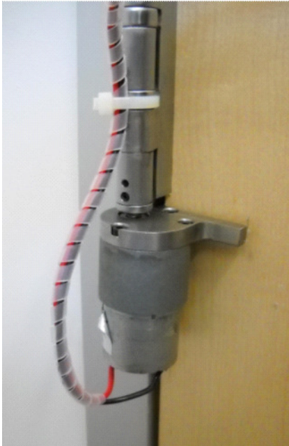
Figure 2. Photograph of Energy Harvesting Unit Mounted to the Door
