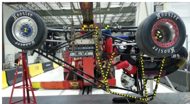
Figure 1. Test Vehicle Prepared for Drop Test
