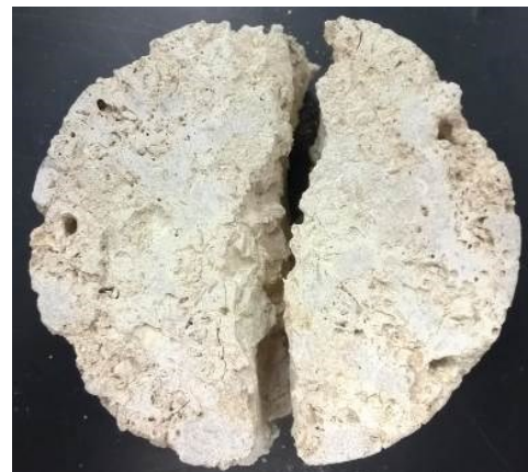
(c) Weathered Specimen (H20) with Central Fracture
