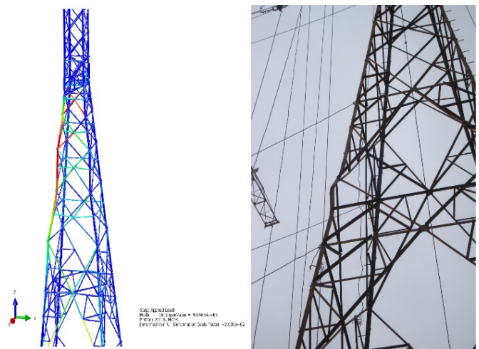
Figure 27. Comparison between Experimental and FE Failure Modes
