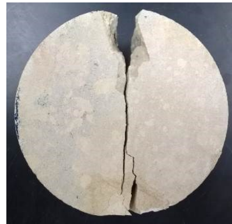
(a) Fresh Specimen (H3) with Central Fracture
