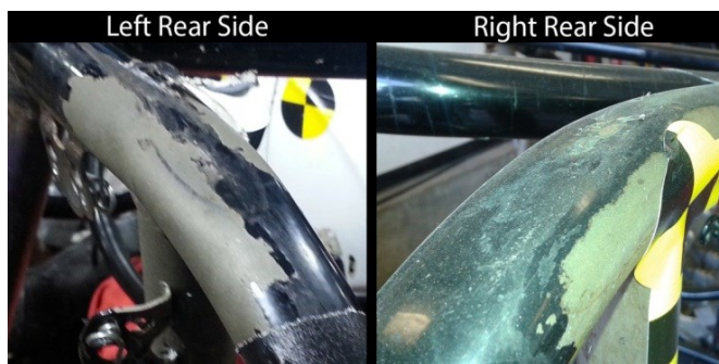
Figure 10. Roll Hoop Damage
