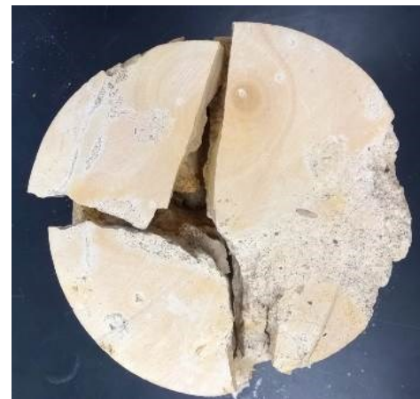
(b) Differentially Weathered Specimen (H18) with Central Fracture and Zone Activation
