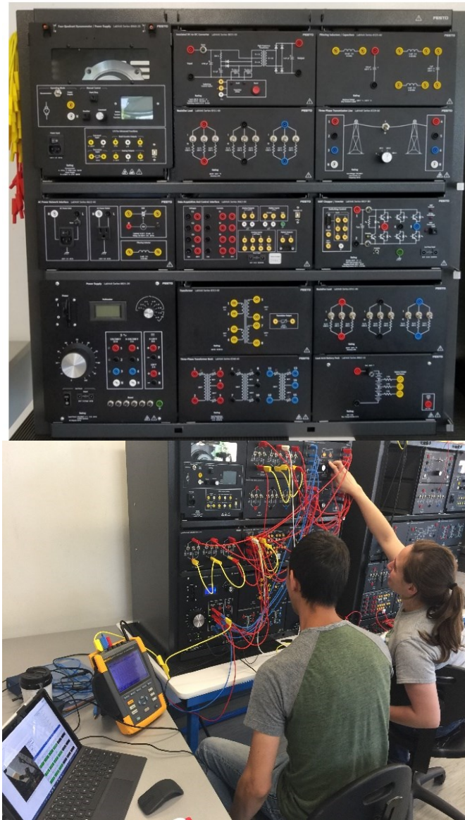
Figure 1. FESTO Smart Grid Technology Training System and students working on the smart grid curriculum. Reprinted with permission.
